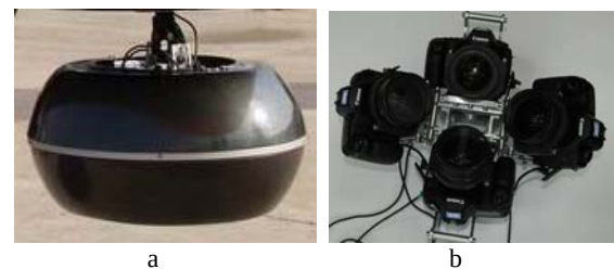
Figure6. a, b the appearance and inside of super-wide-angle camera
