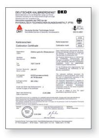
in the German calibration service (DKD), which is controlled by the German federal physical and technical agency (PTB), guarantees compliance of longitude and angle with national norms and regulations. Results of the calibration are listed in a special certificate, the DKD-calibration license. This certificate conforms to all requirements of the DIN ISO series of standards for control of inspection, measuring and test equipment.
